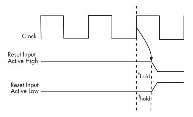
Hold Time for Reset Input Signals
